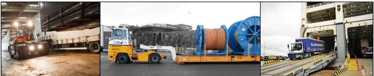
Picture 18 Some of the equipment needed for RoRo-Handling, Terminal Tractor (TT) on each picture, in middle there is the goose neck, TT handling cable reels on a Mafi platform with goose neck. Pictures: Kalmar Global, Mafi and Terberg.
