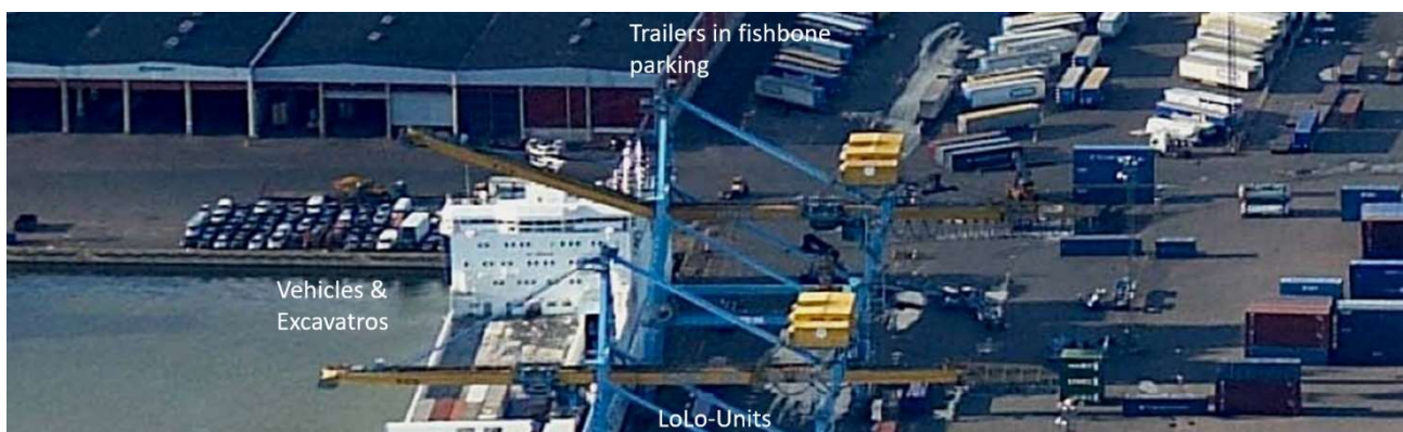
Picture 21 Some RoRo-Cargo groups around Transfennica ConRo-Vessel. The cassettes and mafies are stored in "attack"-position on WH on back of the picture.
