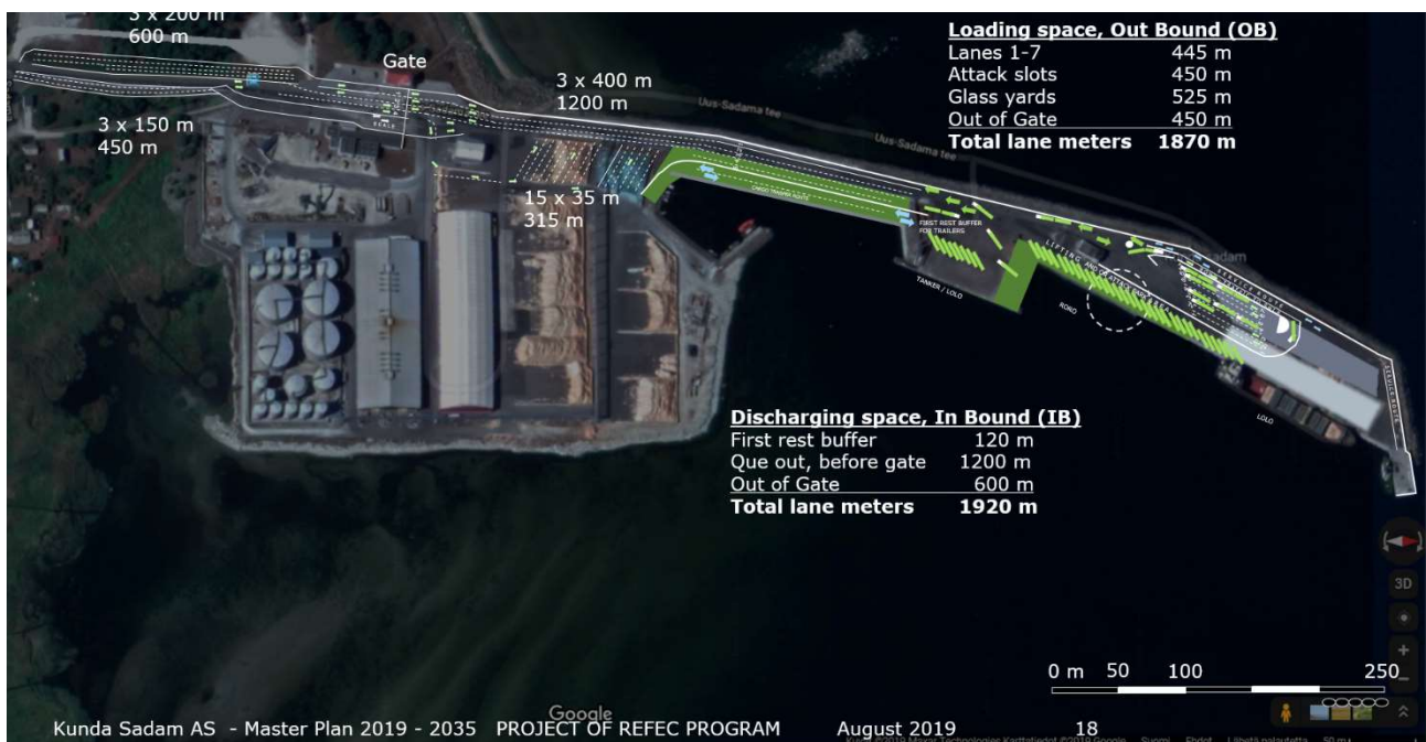
Picture 20 Overall capacity for the RoRo-service has been checked and it seems that it does not yet be adequate for the RoRo-Vessel traffic. The additions have been indicated in picture above, where the left green area and the right one show the berth extension works executed. The root of the pier extension would enable the port to work with other vessels regardless the RoRo-actions at the end. Rebuilding the berth no.3 and larger yard would bring the RoRo-quay area to a sufficient level for twice per day gathering of trucks, both inbound and outbound vehicles
